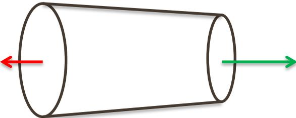
$$\begin{aligned} \oiint \vec{v} \cdot \vec{dS} &= \iiint \text{div}(\vec{v}) d\tau = 0 \\ &= \iint_{\text{entrant}} \vec{v} \cdot \vec{dS} + \iint_{\text{sortant}} \vec{v} \cdot \vec{dS} = 0 \end{aligned}$$
